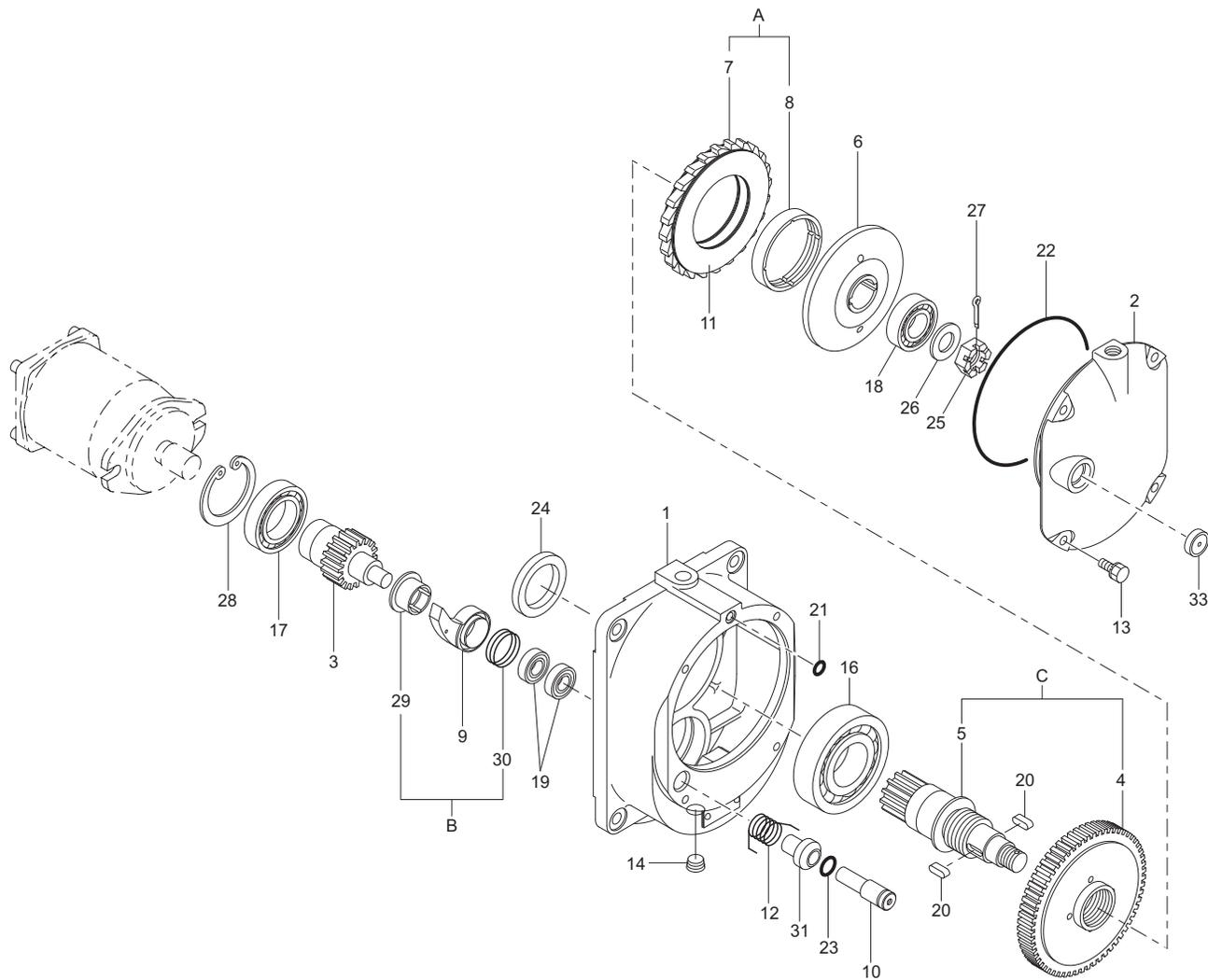
Fig. 11-1-1 HOIST WINCH REDUCTION GEAR ASS'Y
