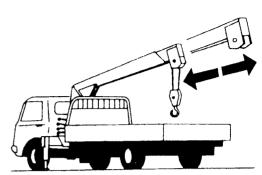
To extend the boom····· Move the lever to push.
