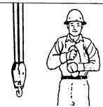
TRAVEL (Both Tracks). Use both fists in front of body, making a circular motion about each other, indicating direction of travel, forward or backward. (For land cranes only.)
