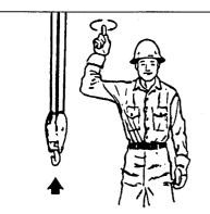
HOIST. With forearm vertical, fore- LOWER. With arm extended downfinger pointing up, move hand in small horizontal circle.
