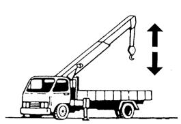
To lower ...... Move the control lever to push. To hoist ...... Move the control lever to pull.
