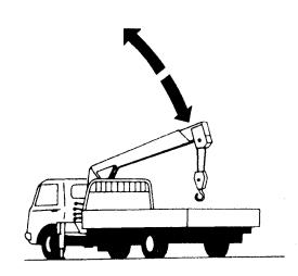
To lower the boom ...... Move the control lever to push.
