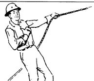
(Telescoping RETRACT Boom). One Hand Signal. One fist Boom). One Hand Signal. One fist in in front of chest with thumb tapping front of chest, thumb pointing out chest.
