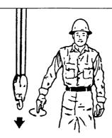
LOWER. With arm extended downward, forefinger pointing down, move hand in small horizontal circle.
