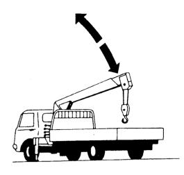
To lower the boom ...... Move the control lever to right.
