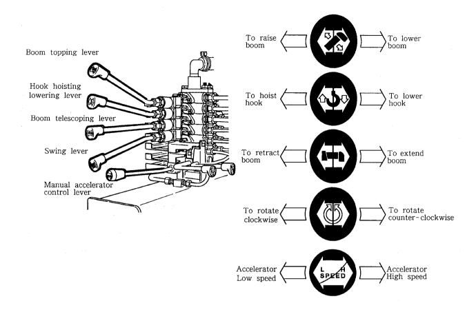
Boom: To lower boom, move lever to right;
