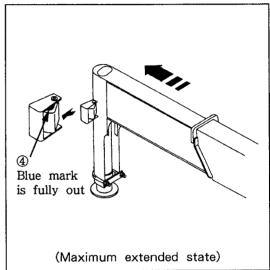
(5) Move the outrigger control lever to push to extend the outrigger cylinders.
