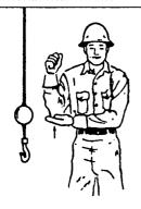
USE WHIPLINE (Auxiliary Hoist). Tap elbow with one hand; then fingers closed, thumb pointing use regular signals.
