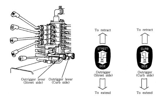
Outriggers: To extend outrigger cylinder, move lever to **push**;
