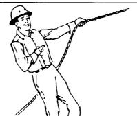
RETRACT BOOM (Telescoping Boom). One Hand Signal. One fist Boom). One Hand Signal. One fist in front of chest, thumb pointing outward and heel of fist tapping chest.
