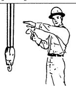
MOVE SLOWLY. Use one hand to RAISE THE BOOM AND LOWER THE give any motion signal and place LOAD. With arm extended, thumb other hand motionless in front of pointing up, flex fingers in and out hand giving the motion signal. (Hoist slowly shown as example.) desired.
