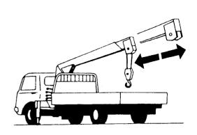
To extend the boom ...... Move the lever to right.
